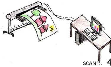
Align the middle of drawing with the center of plotter feeder. Stick drawing into the plotter face up and make sure the plotter catches the end of paper. Press SCAN on computer. In case computer fails, restart program or computer. Release drawing with the lever on the back. There is no need to enter any information or press any buttons on scanner.
